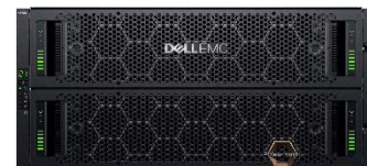
ME4084 SAN/DAS ARRAY (84 drive) 2.5” drive slots, 5U
